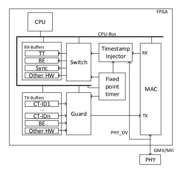
Fig. 2. Overview over the architecture of the FPGA implementation
