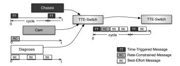
Fig. 1. Prioritising and time-triggered media access in time-triggered Ethernet
