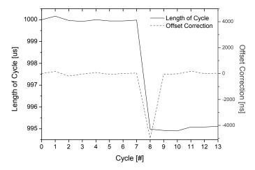
Fig. 4. Behaviour of the Hardware Implementation of the Synchronisation Protocol
