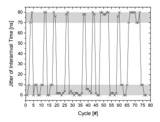
Fig. 3. Jitter of time-triggered messages (measured using interarrival time)
