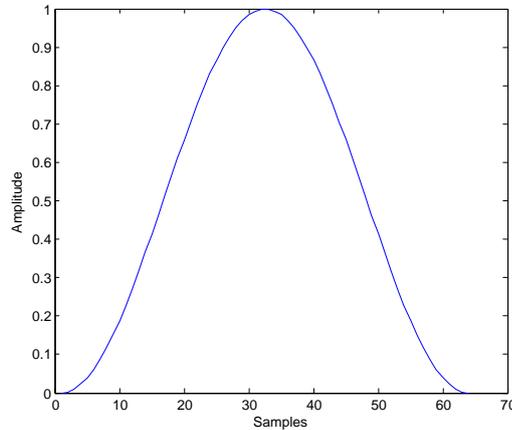
Figure 3: Hann Window with a width of  $N = 64$  samples
