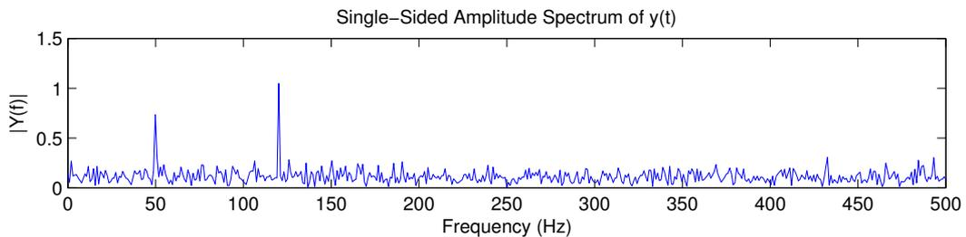
(c) Fourier transform of figure 2(b), showing spikes at 50 Hz and 120 Hz.
