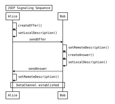
Figure 3.1: Alice establishes a WebRTC connection to Bob by following the JSEP signaling sequence using an arbitrary channel to transmit the offer/answer messages.
