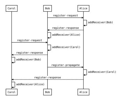
Figure 4.2: Bopcast sequence diagram showing the process of forming a group of peers
