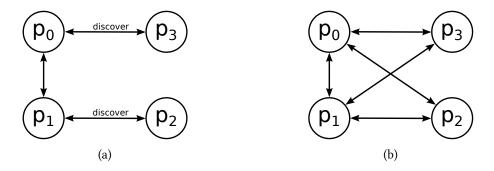
Figure 4.4: When two peers  $p_2$  and  $p_3$  join the network in parallel – each using a different bootstrap peer – as seen in (a) the current Router implementation may lead to a network as outlined in (b) where no full mesh is constructed because the link between  $p_2$  and  $p_3$  is missing.
