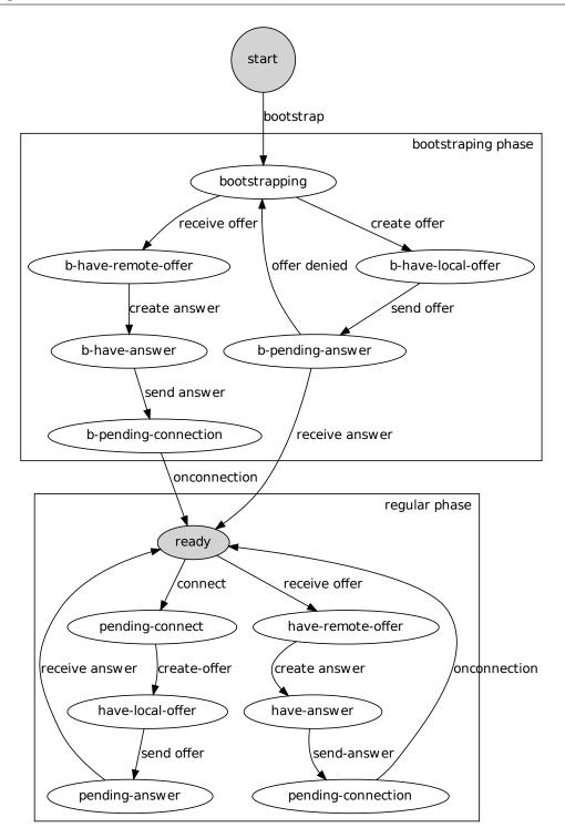
Figure 4.3: The Connection Manager implements a state machine consisting of a bootstrapping and a regular phase. The bootstrapping phase is entered for acquiring an initial connection to an arbitrary peer. After this connection has been established, the regular phase is entered in which additional connections can be established.
