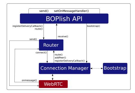
Figure 3.3: Outline of all BOPlish components and their interaction with one another. Each component is strictly defined by a set of API calls and loosely coupled to the other components. This enables us to easily replace parts of the functionality without having to refactor reliant code.
