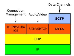
Figure 1.2: The protocol stack of WebRTC is divided into a connection management component for establishing and maintaining connections even across middle boxes, an A/V component and a Data Channel component. Both audio/video data as well as Data Channel streams are encrypted end-to-end using SRTP/SRTCP and DTLS, respectively.
