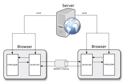
Figure 1.1: Schematic view of a WebRTC connection. The server delivers applications (consisting of HTML, CSS and JavaScript code as well as resources such as images) to all the client browsers. Additionally, the server handles the signaling of a WebRTC connection, therefore serving as a central connection establishment entity. After the inital connection establishment, the server may be shut down.
