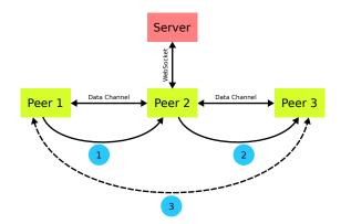
Figure 3.2: Peer 1 wants to communicate with peer 3. Therefore it sends the data via the open Data Channel to peer 2 which in turn routes it to peer 3. The server is not involved in this process at all.
