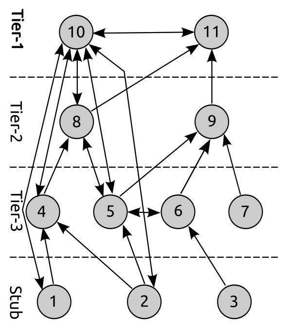
Figure 4: Topology of the test network during the second part of the experiments. [Customer  $\rightarrow$  Provider, Peer  $\leftrightarrow$  Peer]
