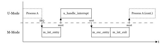
Figure 1: Interrupt dispatching and handling in U-mode
