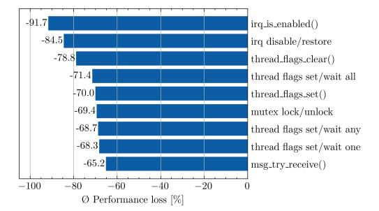
Figure 3: Microbenchmarks: Some API functions of RIOT show a significant performance loss between 92% and 65%.
