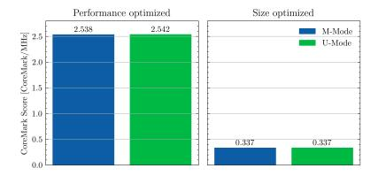
Figure 2: CoreMark Benchmark: Both the performance and size optimized compiler profiles show no significant difference in the CoreMark score.
