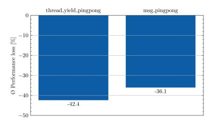
Figure 4: Context-switch benchmark: Performing a context switch, as a result of yielding or blocking IPC mechanisms, is slowed down by up to 42%
