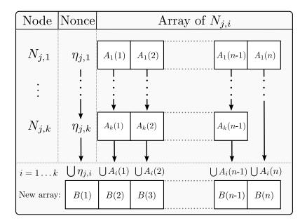
Figure 5.2: MERGING OF NONCES INSIDE A NODE – In a) the received Bloom filter arrays  $A_1 \dots A_k$  of nodes  $N_{j,1} \dots N_{j,k}$  of rank j are united into the new array B starting at its 2nd index position. B(1) holds the united received nonces  $\eta_{j,1} \dots \eta_{j,k}$  in a newly created filter v.
