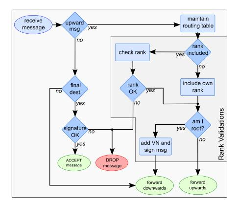
Figure 6.1: PROCESSING OF ATTESTATION MESSAGE IN TRAIL PROTOTYPE
