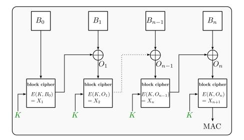
Figure 2.1: CREATION OF A CBC-MAC IN CCM – The first block  $B_0$  is encrypted by a block cipher function E using secret key K. The resulting  $X_1$  is XORed with the second block,  $B_1$ . The resulting output  $O_1$  in turn is encrypted, and so on. The last (truncated) block denotes the MAC.
