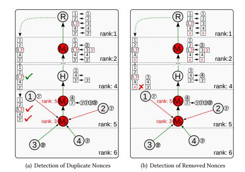
Figure 5.5: NONCE DUPLICATE AND REMOVAL DETECTION – Squares denote array elements, circles denote single nonces. Attacker  $M_1$  copies the nonces from the correct array element to the index of the spoofed rank of  $M_3$ . In a) Nodes check for duplicates and detect the modification. In b)  $M_1$  removes the duplicate nonces. Honest node H detects missing nonces and drops the message.
