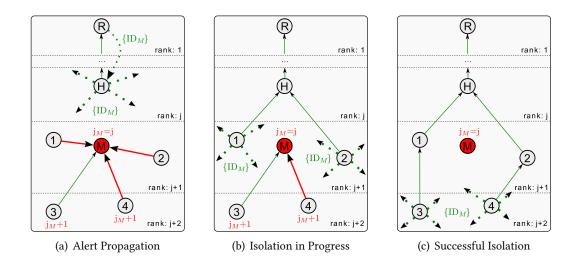
Figure 4.3: ATTACKER ISOLATION FOR RANK REPLAY DEFENSE – Local flooding of the signed alert message  $\{ID_M\}$ . In a) node H receives the alert message from the root and begins its dissemination. b) shows nodes 1, 2 isolating M by correctly selecting H as parent. In c) malicious node M is isolated from topology.
