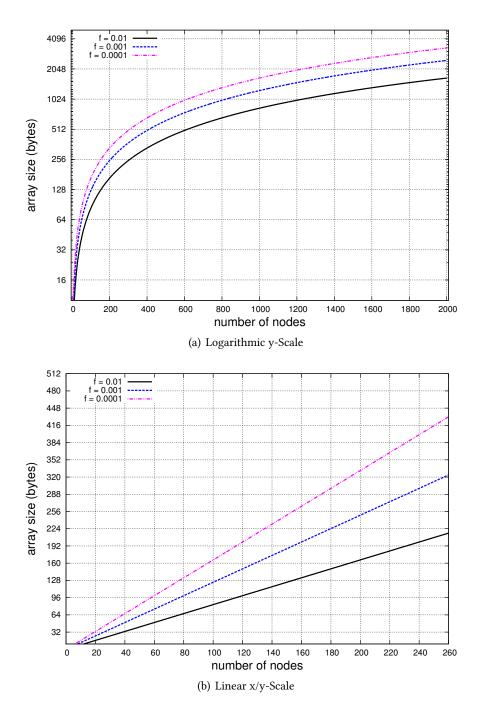
Figure 5.6: TRAIL Compressed Array Sizes for Different Error Rates
