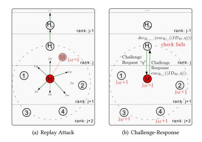
Figure 4.2: RANK REPLAY DEFENSE BY CHALLENGE-RESPONSE – (a) Attacker M replays the rank announcement via multicast thus falsifying the local topology. (b) Its parent  $H_P$ receives the replay as well. The honest node challenges the attacker by sending a random nonce  $\eta$ . The challenge can only be solved if M has a relation with a node of rank  $R_{i,j-1}$ .
