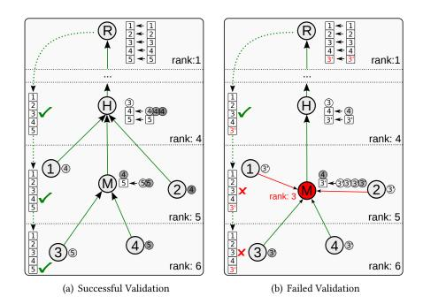
Figure 5.3: PRINCIPLE OF NONCE AGGREGATION IN TRAIL – In a) nonces (circle) and arrays (square) are aggregated in the DODAG. The number denotes the index of the array and thus the rank of the parent. Nodes match their signed nonce at the index that denotes the parent's rank. In b) M propagates a false rank of 3, so that nodes 1 and 2 select M as parent. The verification fails, because nodes cannot match their nonces as they move to the wrong index.
