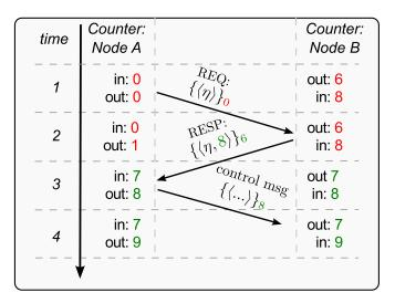
Figure 2.6: SYNCHRONIZATION OF CCM COUNTER – Node A sends a CC request  $\{\langle \eta \rangle\}_0$  to B. The request contains a nonce  $\eta$  and is protected by A's initial counter state (0). B replies with a CC response  $\{\langle \eta, 8 \rangle\}_6$  containing its incoming counter (8) and echoing  $\eta$ . The response is secured by B's outgoing counter (6). Node A resets both counter states, so that further communication uses synchronized counter states.
