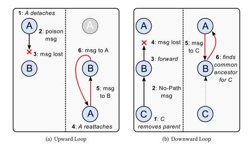
Figure 2.5: FORMATION OF ROUTING LOOPS IN RPL – Figure a) shows a loop due to a lost poison message. An upward message is falsely sent downwards. In b) the loss of a No-Path DAO results in a downward loop. A downward message is falsely sent upwards.
