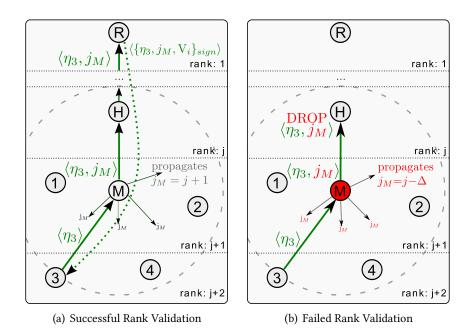
Figure 5.1: PRINCIPLE OF TRAIL RANK VALIDATION – Node 3 sends a nonce,  $\eta_3$ , to M for rank validation. In a) M announces its true rank. The message is signed by the root and thus validates M's rank. In b) M spoofs its rank by  $\Delta \ge 0$ . Since H's rank  $j_H \le j_M$ , the message is dropped.
