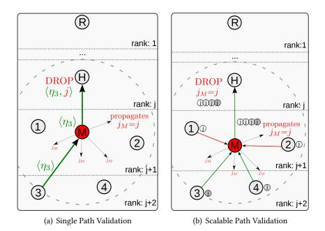
Figure 5.4: RANK REPLAY PROTECTION IN TRAIL – In a) M claims the rank of H and replays the nonce  $\eta_3$  of node 3. H drops the replayed nonce because  $j_M = j$ . In b) children of M send nonces (circles) to validate M's rank j. M replays all nonces to H. Hdrops the nonces due to the equal rank in M rank announcement.
