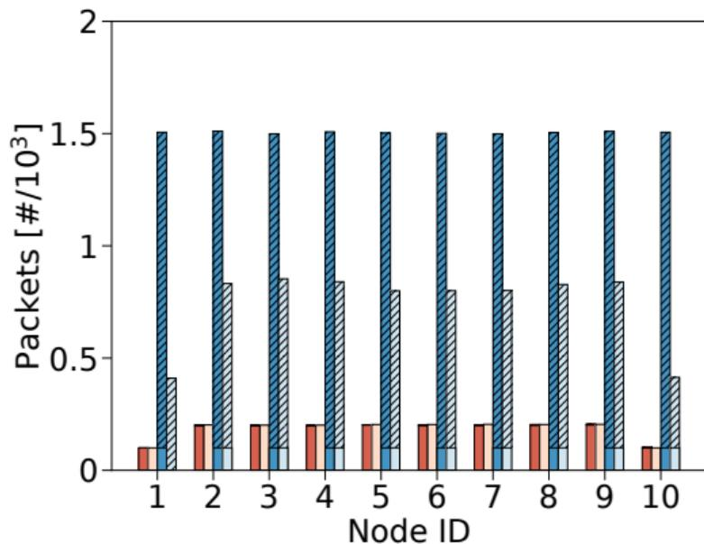
Redundant replications in BT mesh flood the medium with packets
