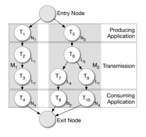
Figure 2: Task graph of two control loops
