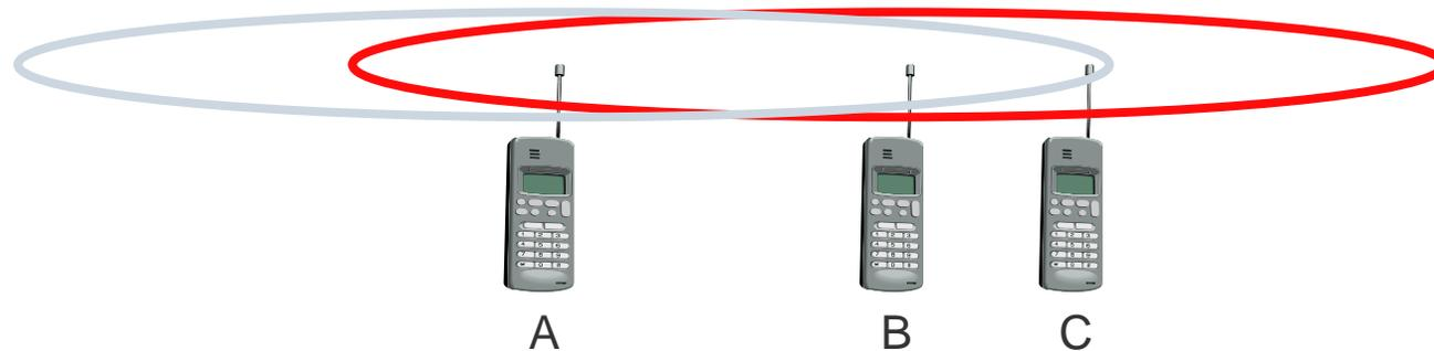
If C for example was an arbiter for sending rights, terminal B would drown out terminal A already on the physical layer
