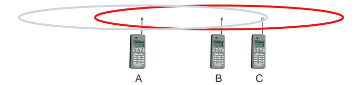
If C for example was an arbiter for sending rights, terminal B would drown out terminal A already on the physical layer
