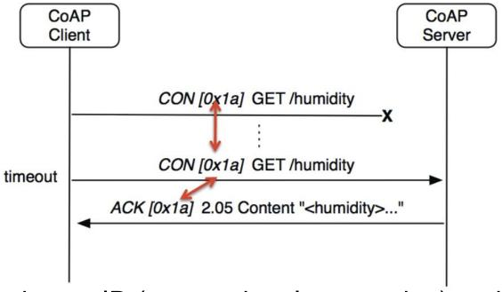
Each message carries an ID (transactional processing) and an optional token (for asynchronous matching)
