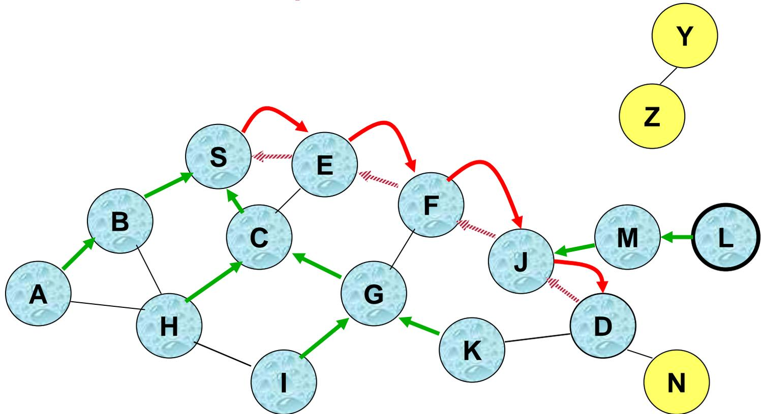
**Forward links are setup when RREP travels along the reverse path**
